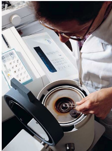
Acid test: Material inspection of a ceramic ball for hybrid rolling bearings at the FAG research centre.
