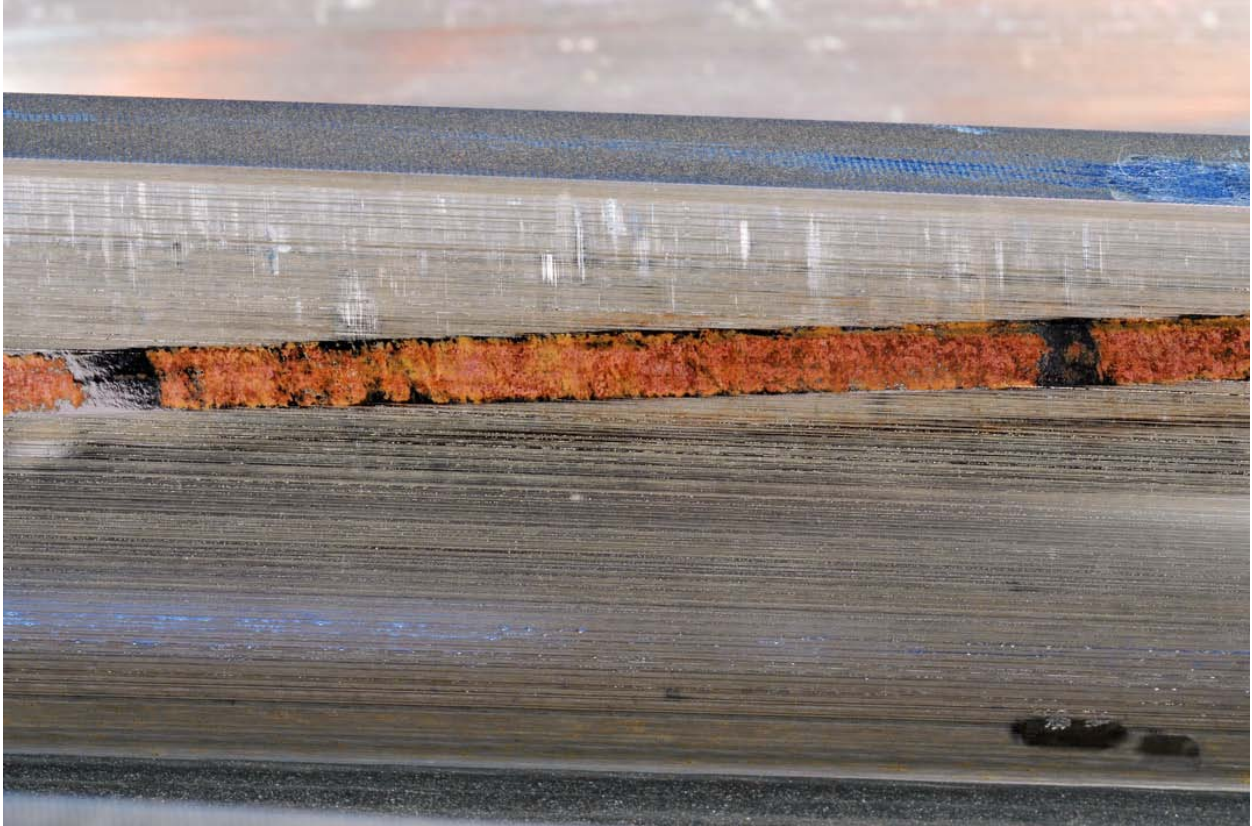
Figure No: 29 (NREL PIX 19851) Scale: 3.2X Component: sun pinion Failure mode: fretting corrosion Failure mode severity: severe Description: Closeup view of fretting corrosion.
